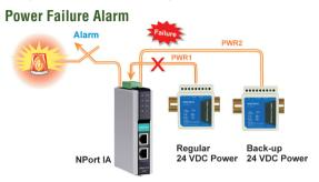
which Ethernet link or power input has failed, or which serial signal has changed. An e-mail warning can also be issued when an exception is detected. These functions are valuable tools that enable maintenance engineers to react promptly to emergency situations
